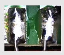
Through hole device to pcb
