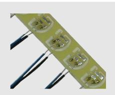
Laser soldering Flex foil
